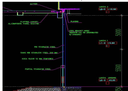
Gambar 39. Potongan Frameless Sumber : PT. Infotech Multifacade Integra Shop Drawing Proyek Sahid Eminance Ciloto;2016
