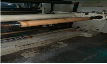
1. As Shaft Unwinder belum dipasang core disisi bagian kiri dan kanan
