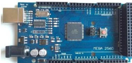
**Gambar 2.4** Arduino Mega 2560
