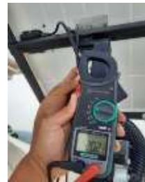
Gambar 3. 19 Pengujian Panel Solar Cell
