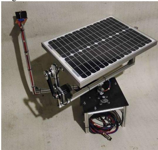
**Gambar 3.5 Sistem Mekanik Dual Axis Solar Tracker**
