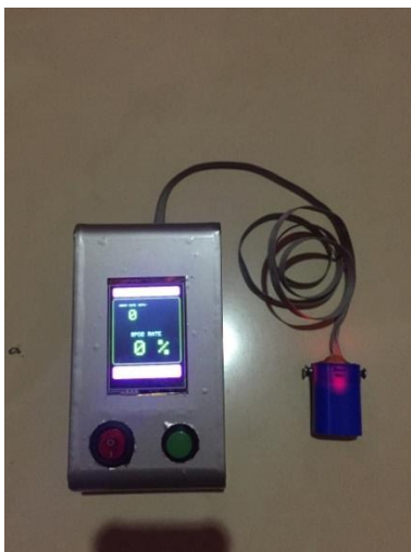
Gambar 9. Modul Pulse Oximetry
