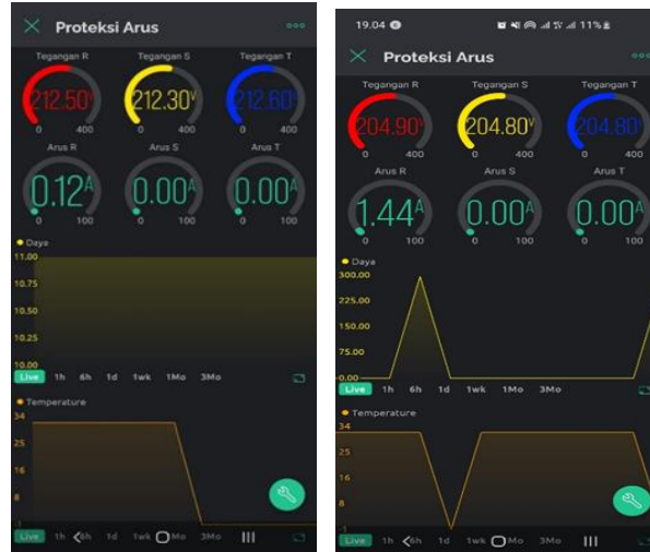
Gambar 9. Tampilan monitoring arus
