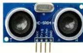
Gambar 2.2 Sensor Ultrasonik
