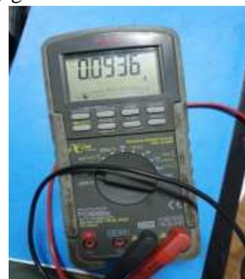
Gambar 3.1 Multimeter
