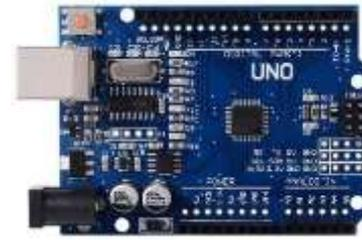
Gambar 1. Arduino Uno Atmega 328P
