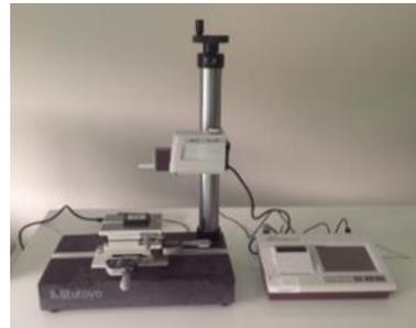
Gambar 3. Roughness Measuring Machine (SJ-411) Mitutoyo
