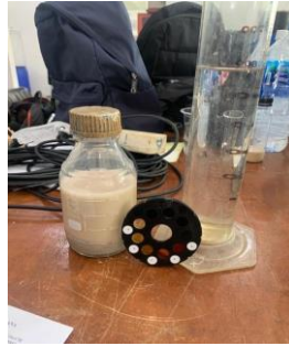
Gambar 2. Pengujian Kadar Organik Agregat Halus
